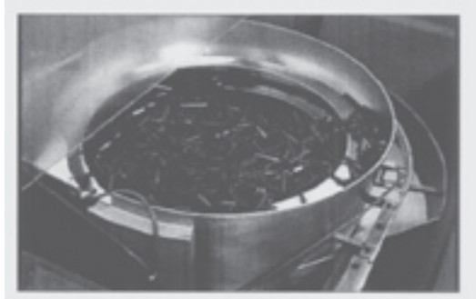
Connector covers fed into a vibratory bowl
