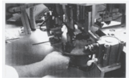
Loading cable on Station 1 of SATA Cable Connector Assembly Machine
