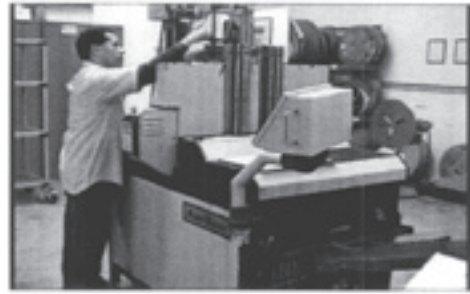
The printed cable reel is mounted on the AutoTerm machine, together with the taped IDC connector and cover reels.
